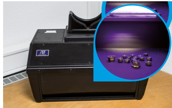
Dark chamber with integrated UV light sources and white light
