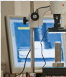
Microscope de mesure Hitec Hitec- Measuring microscope
